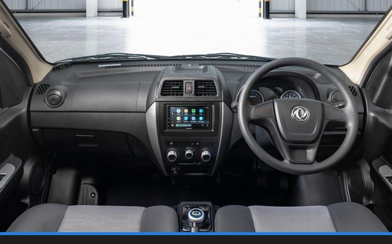
The well-equipped cabin is fitted with two adjustable seats in grey fabric, with co-ordinating black and silver dash. The instrument panel shows you the available battery charge so you can predict when they'll need to plug in next. The 6.8-inch screen with Android Auto<sup>™</sup> and Apple CarPlay<sup>®</sup> is set in the centre of the dashboard. Your reversing camera video will display on this screen when activated. The DFSK EC35 comes with electric windows as standard and a manual handbrake.
